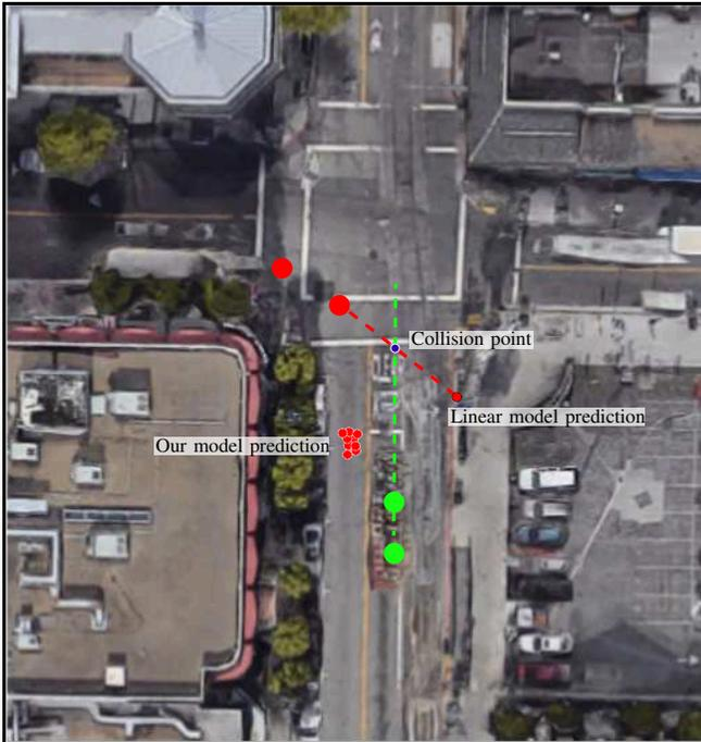
Fig. 6: A comparison to the linear model. The big red circles indicate the position of an oncoming car at  $t$  and  $t+1$ . Under the linear model, it is expected to collide with our vehicle. Our model corrects for this error using the motion prior.
