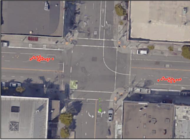
Fig. 4: Vehicle motion predictions at intersections. The green circle represents the query position and velocity at time  $t$ . The red icons represent the distribution of predicted samples at  $t + 5$ . Note that the road ahead is a one-way route in opposite direction. Our prior implicitly capture this information without any manual annotation.
