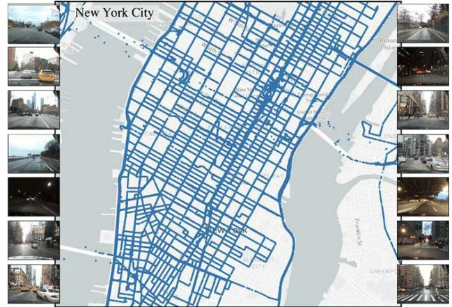
Fig. 5: Dataset used to evaluate the method. We have collected over 10M images in San Francisco and New York using dashcam-mounted mobile phones. These images were used to perform large-scale structure-from-motion to reconstruct accurate vehicle trajectories in the city over a period of several weeks.
