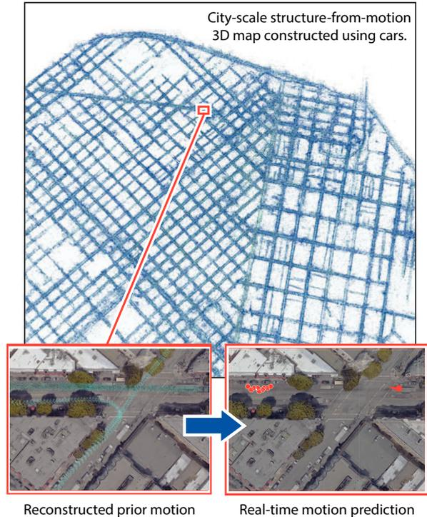
Fig. 1: Our system can accurately predict the future position of a vehicle based only on the previous motion in the area. This prior motion was crowd-sourced by a fleet of mobile-phone-equipped cars.
