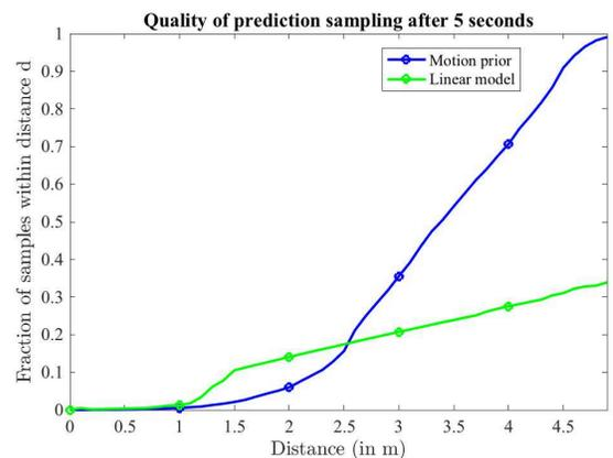
Fig. 7: The average fraction of the predictive distribution within distance  $d/m$ . As the predictive distance increases, the motion-prior model quality increases rapidly, while the linear-motion model is slow to improve.
